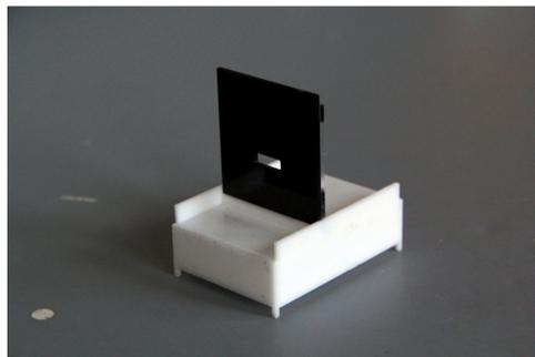
Remove the protective paper from the clear acrylic and glue it to the inside of the crossbar, then glue the black window piece onto the clear, resting on top of the crossbar as shown.
