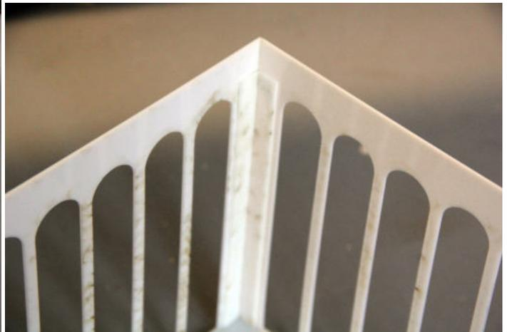
Start by gluing the rear and side wall to the EDGE of the base, which is the 1/8" thick solid piece. The 1/16" same size piece is the roof. Glue in the corner strips, the widest ones facing the rear and front.
