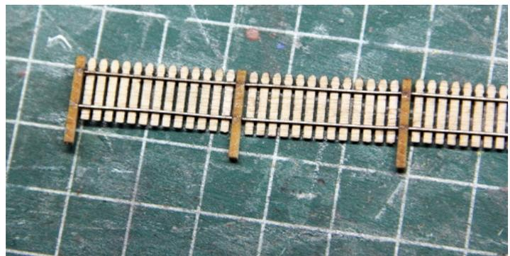
Peel off the backing paper and mount the self-adhesive runners to the (back) of the fence boards, the overhang should be the same in both ends.
