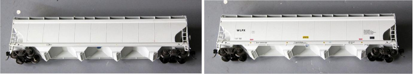
Carefully remove all print from the decal side of the car, using fine (600 grit) sandpaper. The other side of the prototype car has no graffiti, so here you remove only the car number (or the reporting marks if you don't have a WLPX car)
