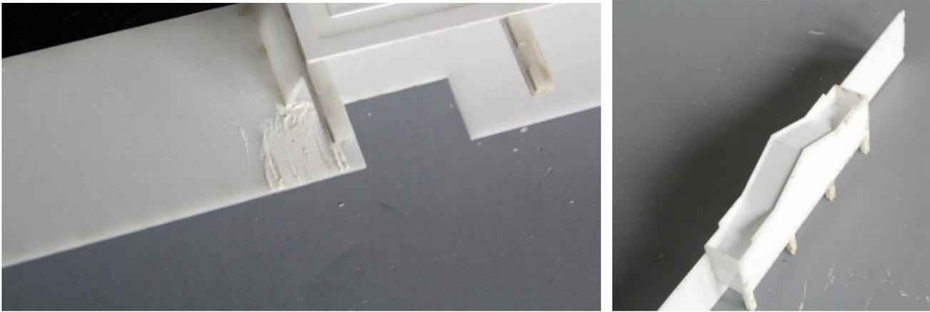
When the Model Filler has dried, sand the joints with 120 grit sandpaper until the surface is even, then sand with 600 grit sandpaper to get a nice smooth surface.
