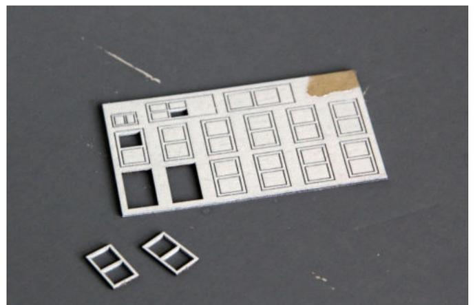
Test fit the house on the floor. Cut the windows and doors out of the sprue and clean them for any burrs.
