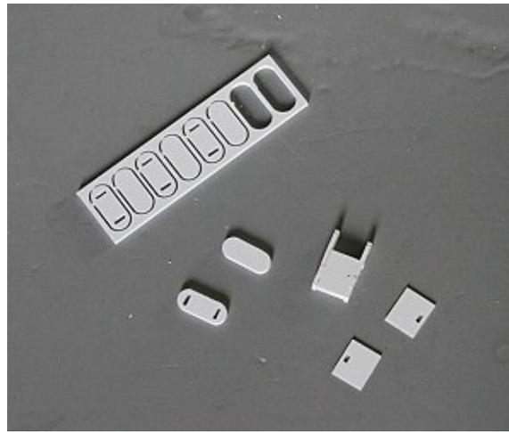
Glue the front piece on so the small hole is to the right when viewed from the front. Glue on the other side and front piece. Glue the two oval pump tops together (lamininate).
