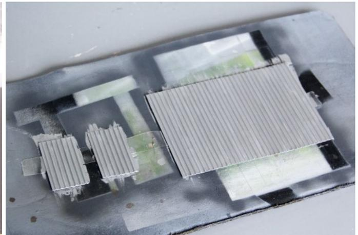
Mount masking tape on the inside of the walls to prevent paint from coming inside if you airbrush. Airbrushing is recommended, so you won't fill the mortar lines up with paint. Also mask the big roof except the side boards. The glue won't stick on painted surfaces. Paint the metal roof an aluminum or stainless-steel color.
