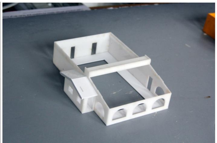
Glue the side boards to the small roof and also to the large roof (not shown). Then glue the top wall in place.
