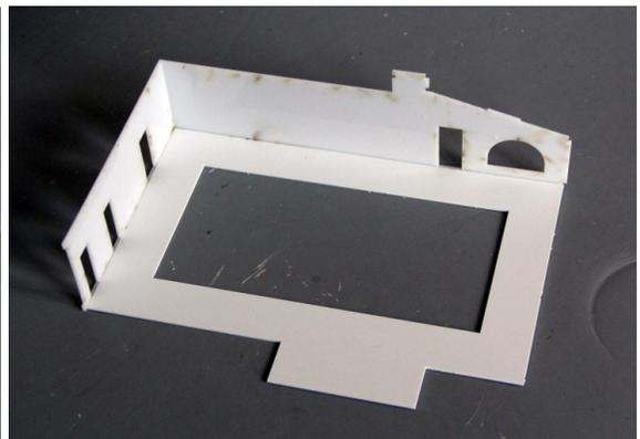
Glue the rear wall and the right-side wall together, then glue the base plate to the INSIDE of the walls
