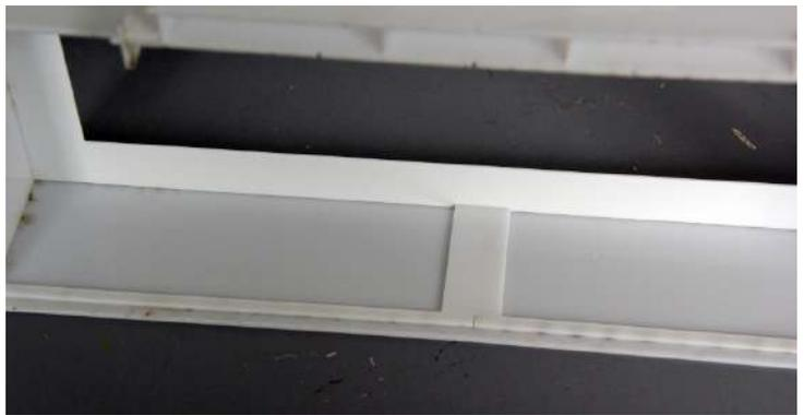
Cut the roof support strips from the sprue, align them with the top of the joint support and glue them on all the way around the walls.
