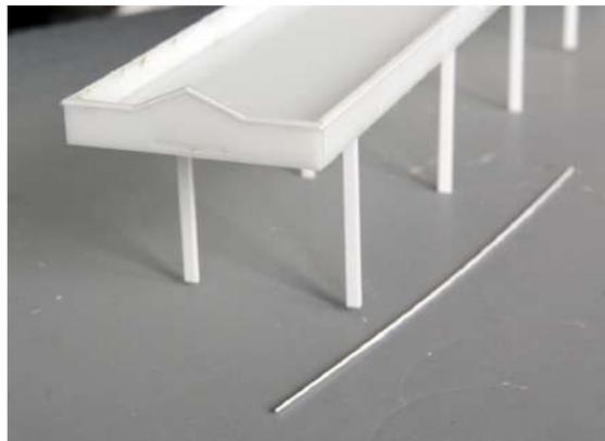
Glue the legs on, the long side perpendicular to the length of the canopy as shown. Take care that the legs are 90° in both directions. Then glue on the thin trim strips around the top edge.
