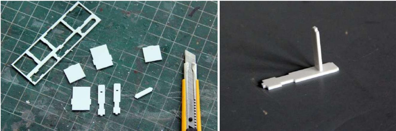
Cut the parts out of the sprue and clean them for any burrs. Glue the small piece into the hole in the side piece.
